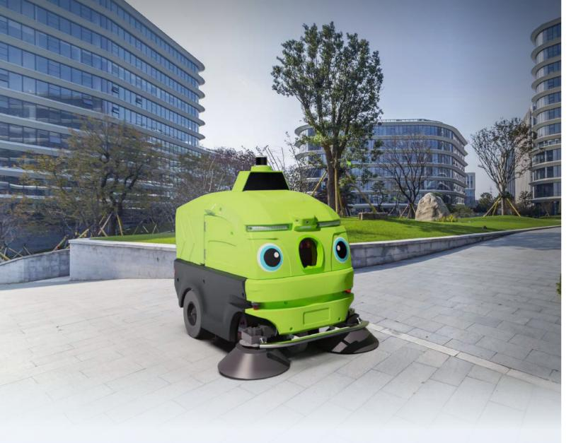
The Greendorph Auto sweeper YJ130 is a fully autonomous outdoor sweeper featuring a primary cleaning system enhanced by three auxiliary functions: suction, airflow-assist, and misting spray. Delivering over 95% cleaning efficiency, it operates continuously for 6–8 hours – ideal for large-area outdoor sanitation across parks, industrial campuses, sidewalks, schools, and similar environments...
