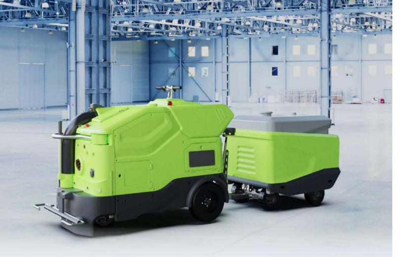
**The Greendorph Omniclean YJ80** redefines versatile cleaning with its semi-autonomous operation. This multi-functional unit adapts to your needs through three intuitive control modes: manual rideon for normal tasks, auto-follow me for effortless operation, and towed traction for extended coverage.
